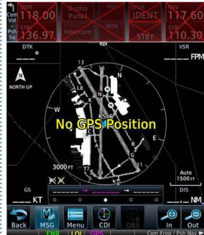
If data fields become invalid, the GTN typically annunciates the failures with a large red X, as shown.
